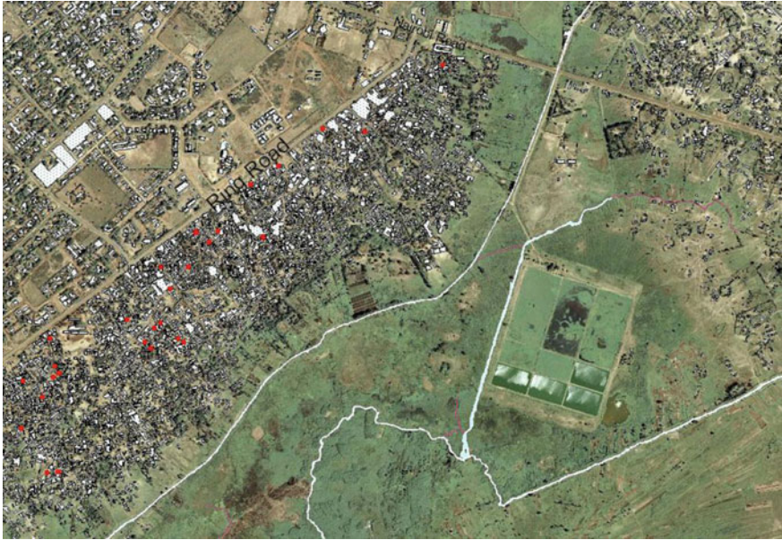
Fig. 15.5 Informal waste dumping locations ( dotted red on the online digital version ) plotted on Map of Nyalenda (Kisumu, Kenya). GNSS could be useful in providing these locations. Source Opande (2008)
