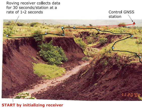
Fig. 5.10 Monitoring of the extent of erosion using the stop-and-go positioning method. The triangle indicate the control station while the circles indicate the positions occupied by the roving receiver. Initialization has to be done at the first station and a lock on four or more common satellites maintained. The advantage over the fast-static approach in Fig. 5.9 is the shorter occupation time (e.g., 30 s compared to 2–10 min). The disadvantage is the loss of lock to the satellite and having to re-initialize
