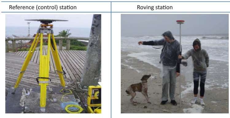
Fig. 12.4 Left , Base station in Matinhos. Right , Real-time GNSS shoreline monitoring. A roving GNSS receiver is used to provide shoreline's location-based data relative to the reference station whose position is known using one of the rapid positioning techniques discussed in Sect. 5.4.5. Source Goncalves (2010)
